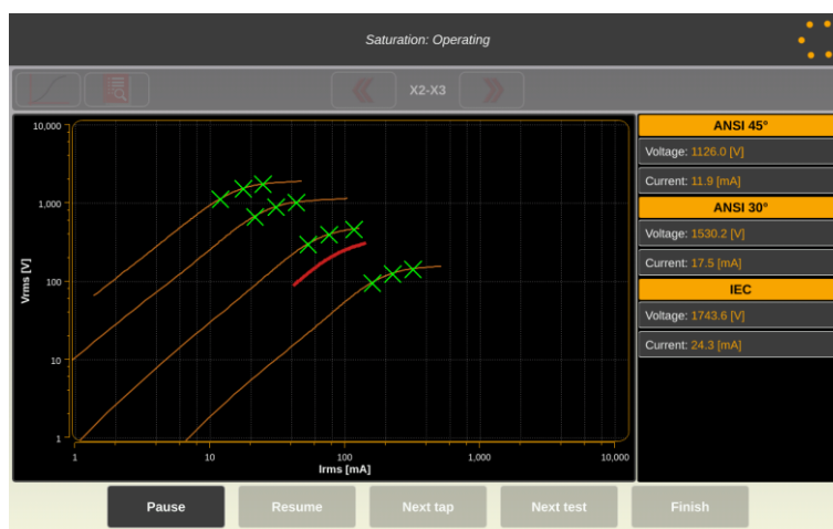
Figure 7-17. Saturation test in progress
