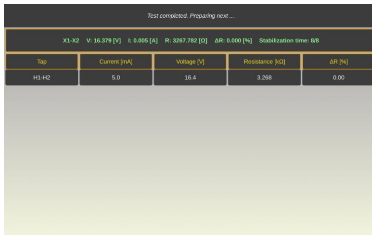
Figure 7-48. Winding resistance results, primary side
