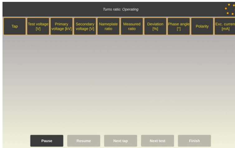
Figure 7-39. Turns ratio test in progress
